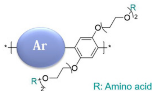
Figure 1: Common structure of synthesized semiconductive copolymers
